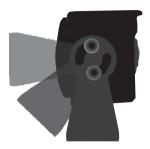
Fasten the camera in a suitable location surface-mounted camera. The bracket can be adjusted in several positions with 4 small screws.
